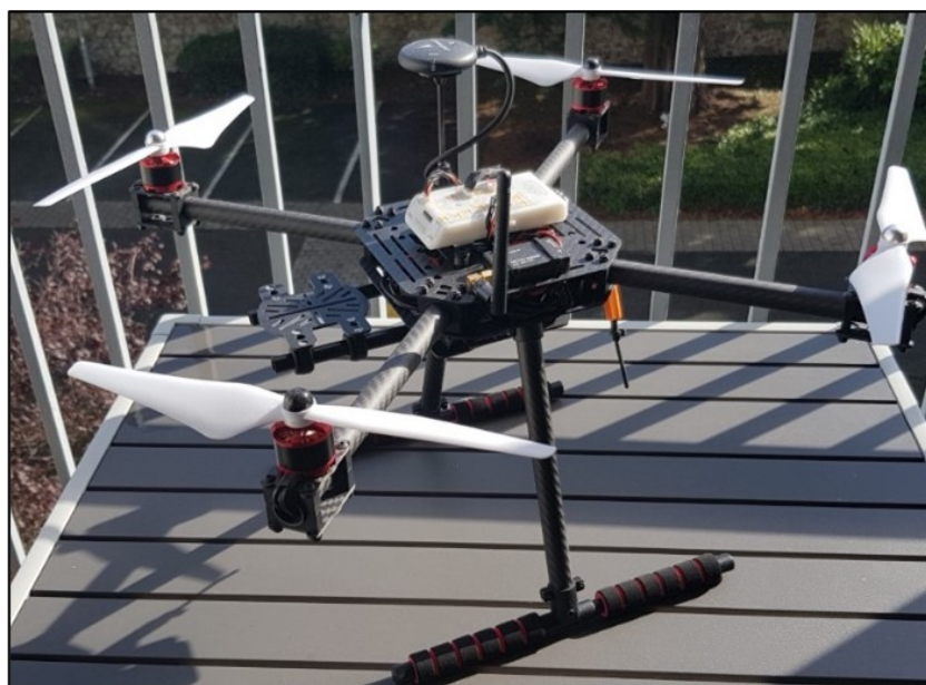
Figure 1. A typical quad rotor helicopter drone, constructed for autonomous flight research.
