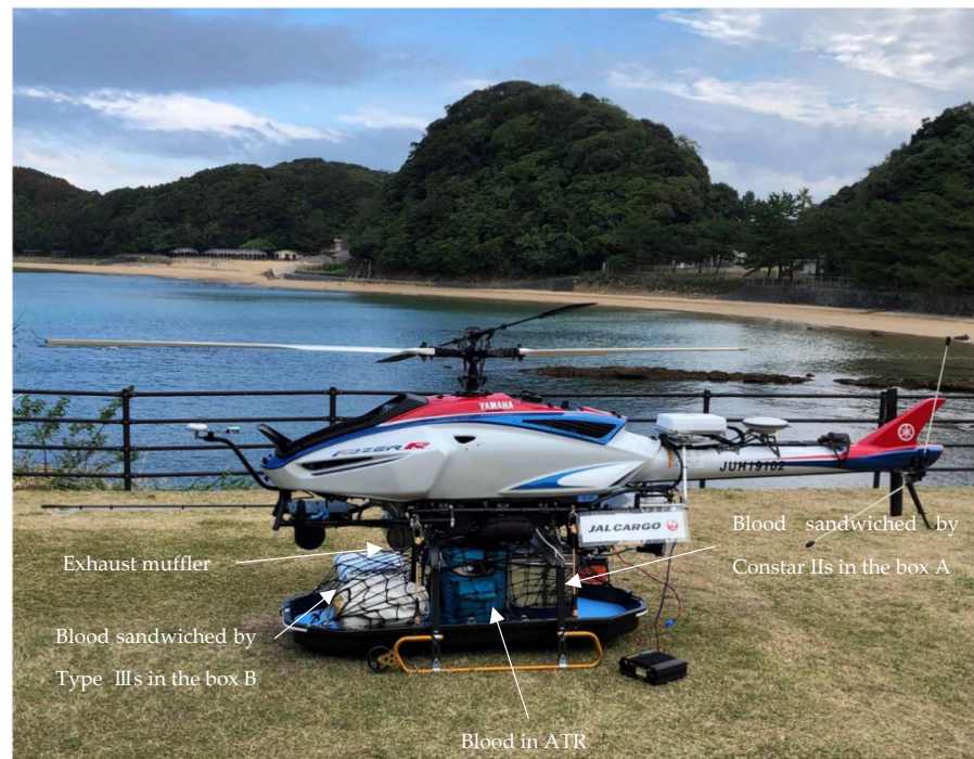
Figure 4. Industrial uncrewed helicopter (FAZER RG2) at the coast of Sasebo City just before the flight to Arikawa port.
