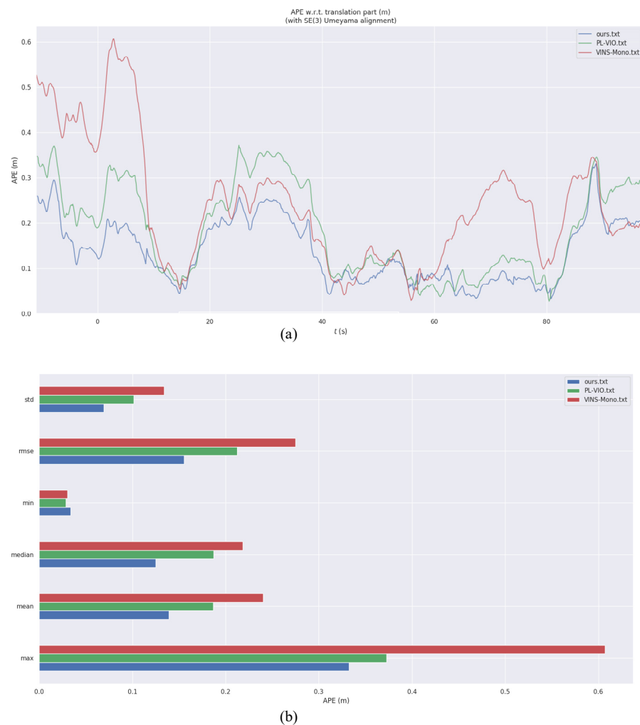
Figure 15. The real-time errors of the three algorithms in V1_03_difficult. (a) the real-time absolute pose error in V1_03_difficult. (b) shows the root mean square error, median error, mean error, extreme error and sum of squares of error of the three algorithms.
