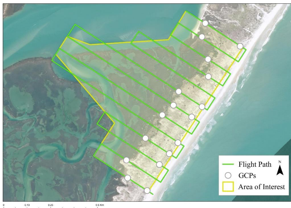
Figure 4. Example flight mission design for Site 3 (Masonboro Island, NC, USA) showing the area of interest for a collection, the LiDAR flight paths generated in ArcGIS Pro and uploaded to Ground Station Pro, and the ground control points (GCPs) used for georeferencing. The fixed wing multispectral flights covered the exact same area of interest and were implemented in eMotion 3.
