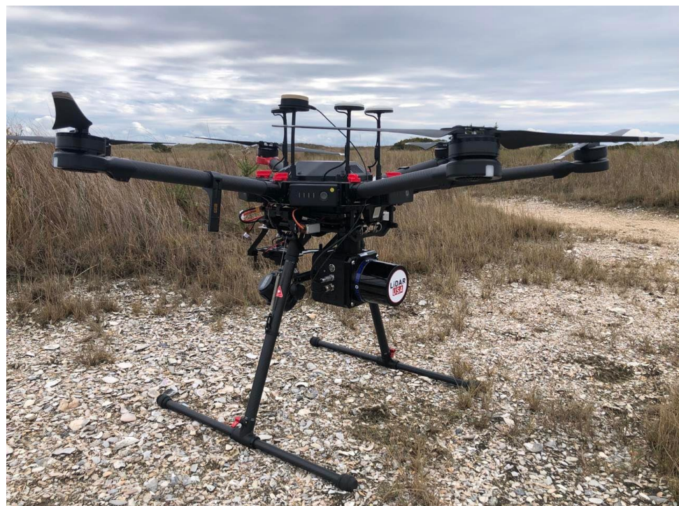
Figure 3. The DJI Matrice 600 Pro (M-600 Pro, manufactured by DJI, Beijing, China) equipped with a LiDAR USA Quanergy M8 LiDAR sensor was used in the study (photo by N. Pricope). The M600 Pro is a six-armed rotocopter with an onboard A3 Pro flight controller and Lightbridge 2 HD transmission system capable of reaching a maximum speed of 65 kph in windless conditions.
