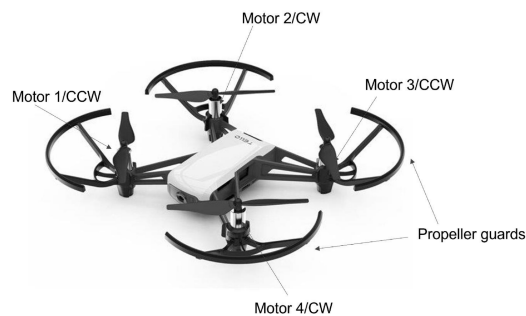
Figure 6. Quadrotor UAV structure [39].
