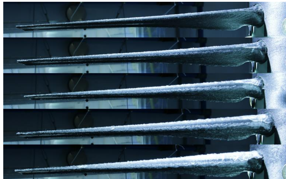
Figure 8. Photographs showing the ice evolution on the rotor blade during 5 time intervals; T_{\infty} = -12\text{ }^{\circ}\text{C} , \Omega = 4950\text{ RPM} , MVD = 800\text{ }\mu\text{m} and \lambda = 80\text{ g/m}^2/\text{h} .
