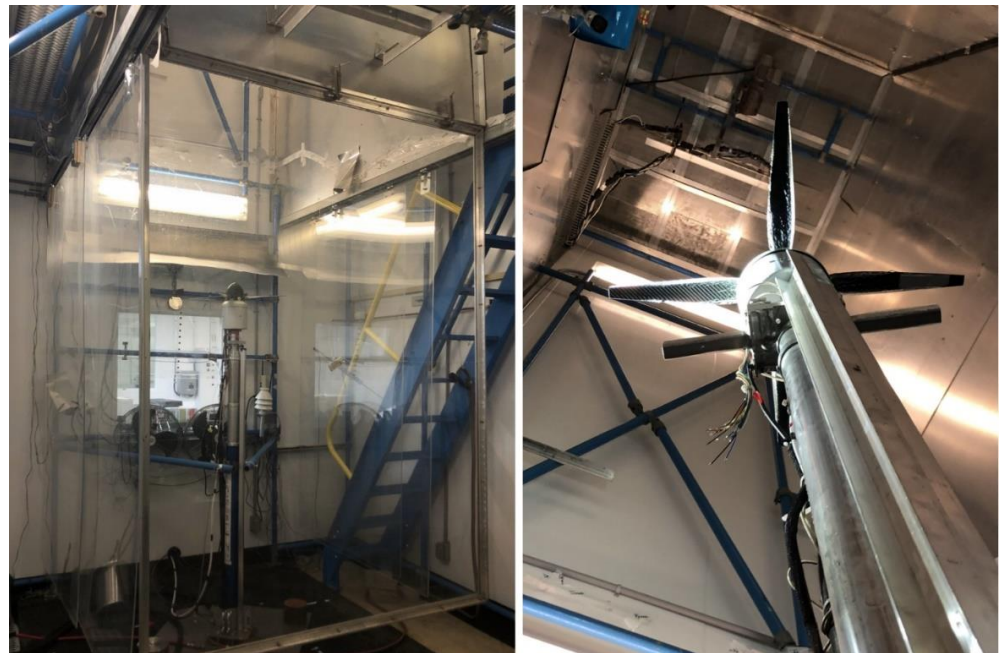
Figure 1. Photos of the experimented rotor system placed inside the cold chamber.
