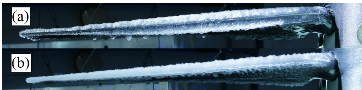
Figure 20. Photographs of blades after icing tests at 4440 RPM, 800\text{ }\mu\text{m} , 0.5\text{ g/m}^3 ( 67\text{ g/dm}^2\cdot\text{h} ): (a) -5\text{ }^{\circ}\text{C} and (b) -12\text{ }^{\circ}\text{C} .
