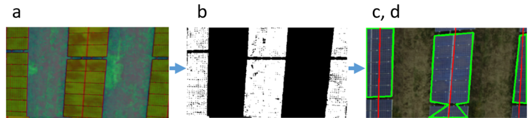
Figure 5. Pipeline for PV module detection from RGB images: (a) transformation into HSV space; (b) binarized image; (c,d) segmentation, regression line extraction and clustering, PV midline estimation.
