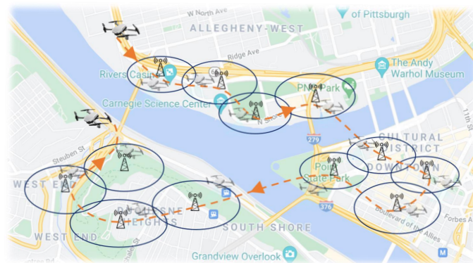
Figure 1. An illustration example: A UAV is dispatched to collect data from a series of ground IoT nodes for scenarios such as fire/flood monitoring, intelligent farming, air quality sensing, etc.
