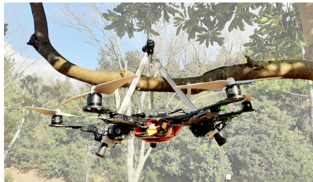
Figure 11. Docking on a non-straight tree branch.
