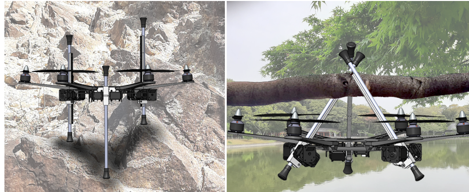
Figure 1. Illustrations of the concepts of adaptive airframe leveling (left) and aerial docking (right) using the proposed manipulator system.
