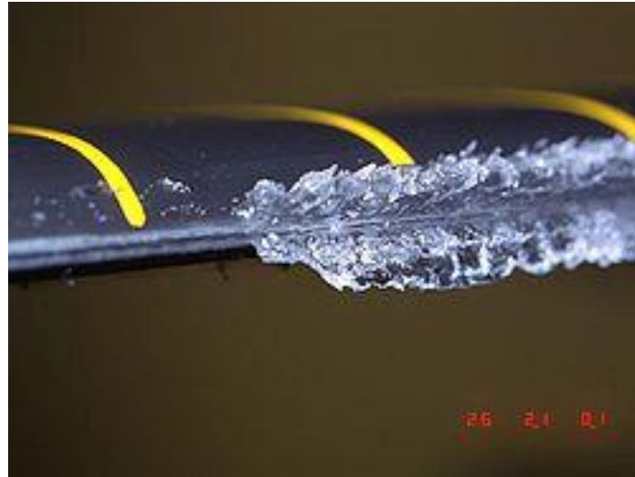
Figure 10. Example of icing on a drone wing (source: NASA [65]).
