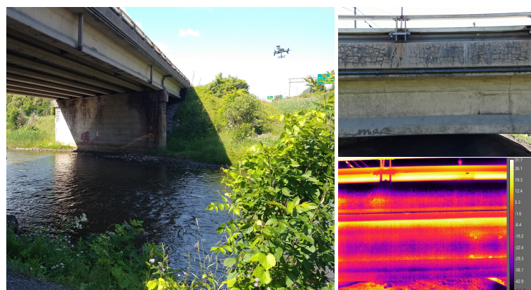
Figure 1. Nondestructive inspection of a concrete bridge using a multi-sensor drone. The left image shows a visual inspection being performed with a drone equipped with multi-modal camera, and the right images show an example of the inspection results: top right image shows the output from the visible camera, and bottom right image shows the correspondent output from the thermal camera.
