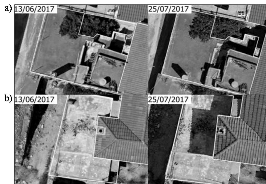
Figure 14. Two examples of commission errors in the case of two different buildings. (a) without shadows at both time-steps and (b) with shadows at the second time-step.
