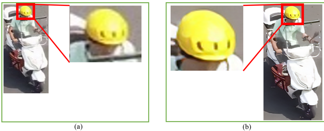
Figure 11. The difference between with and without ESRGAN. (a) shows the original image as well as the enlarged helmet area. (b) is the reconstructed image with the helmet area enlarged.
