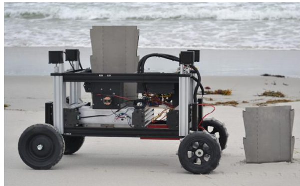
Figure 22. Romu, an autonomous robot capable of carrying sheet piles and driving them [130], reproduced with permission from Melenbrink et. al., Autonomous Sheet Pile Driving Robots for Soil Stabilization ; published by IEEE, 2019.
