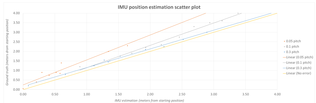
Figure 12. IMU measurements vs. ground truth for various pitch values, including linear trendlines and a no-error line for reference. Note how lower pitch values result in greater errors, and how the angle between the trendlines and the no-error line increases for slower speeds.
