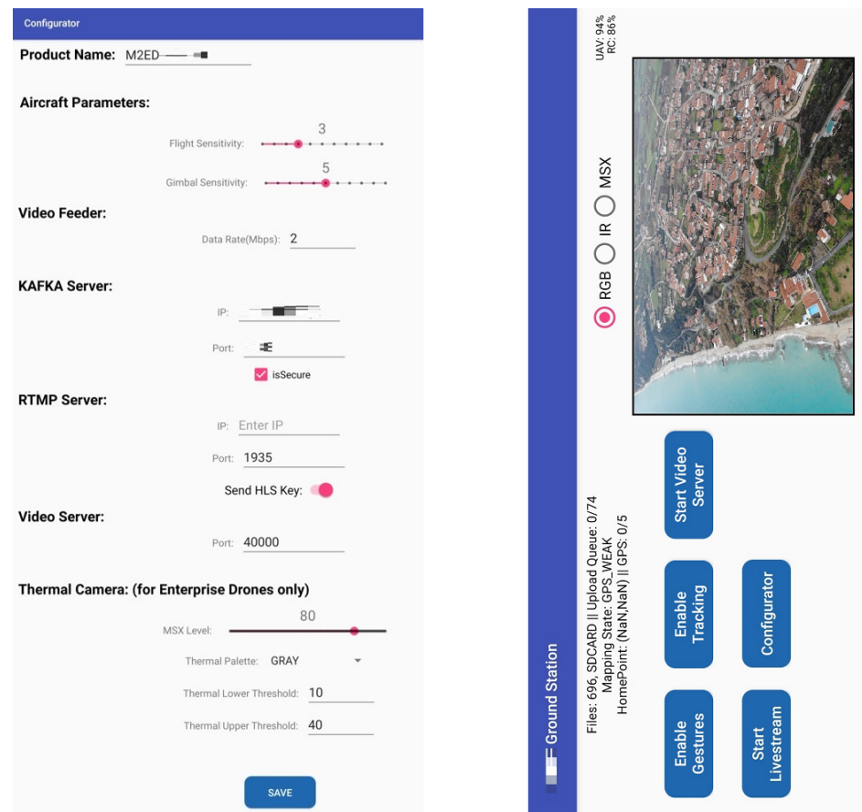
Figure 5. The Android UAV interface app. Left: the app's configurator page, with setting regarding connectivity, gesture command sensitivity, and infrared view display. Right (rotated): the app's main view, showing a live view of the drone's camera feed.
