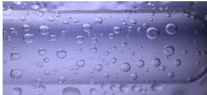
Figure 3. A photograph of the collected water droplets on the glass slide with silicone oil.
