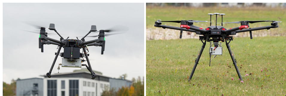
Figure 2. Experimental multicopter platforms with integrated MMT device.
