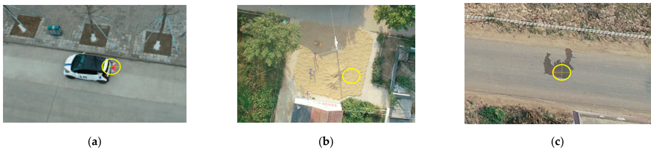
Figure 1. Illustration of anomalous ground control points: (a) car gland; (b) crop gland; (c) vandalism (being cleaned).
