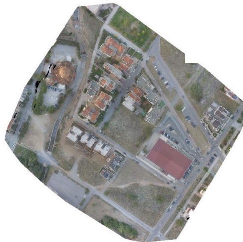
Figure 7. The orthomosaic generated from the data collected (source: Pix4Dmapper).
