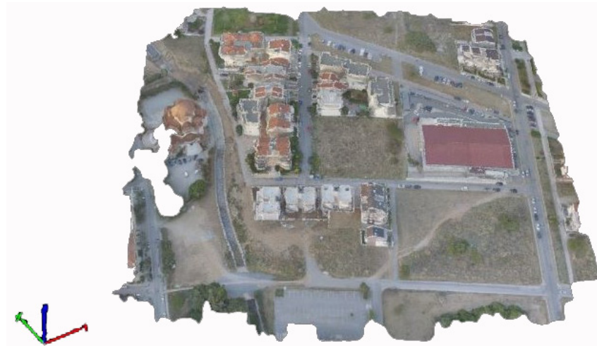
Figure 6. The 3D texture mesh generated from the data collected (source: Pix4Dmapper).
