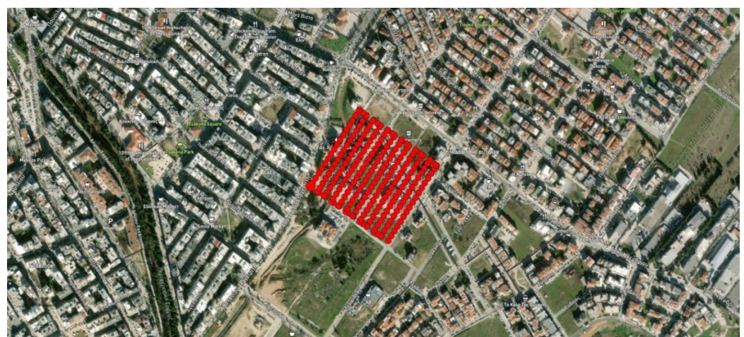
Figure 3. Drone path used for mapping the area (source: Pix4Dmapper).
