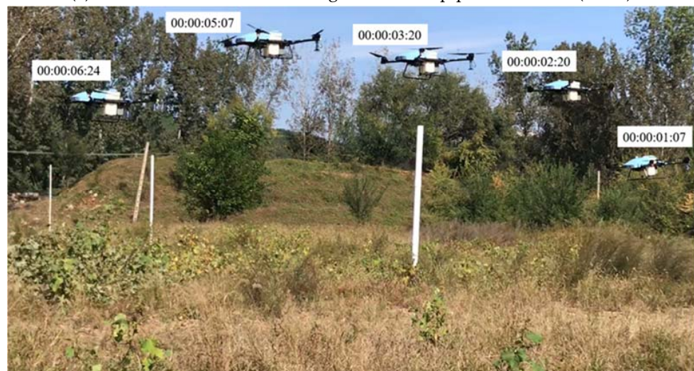
(b) Obstacle avoidance test of large-sized PVC pipe of EAVISION E-A2021 (2 m/s)
