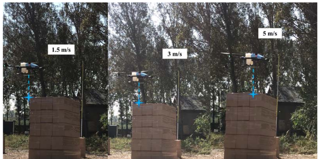
(a) Attitude adjustment points of EAVISION E-A202 at different speeds
