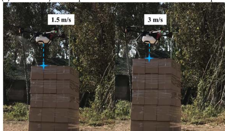
(b) Attitude adjustment points of XAG P80 at different speeds
