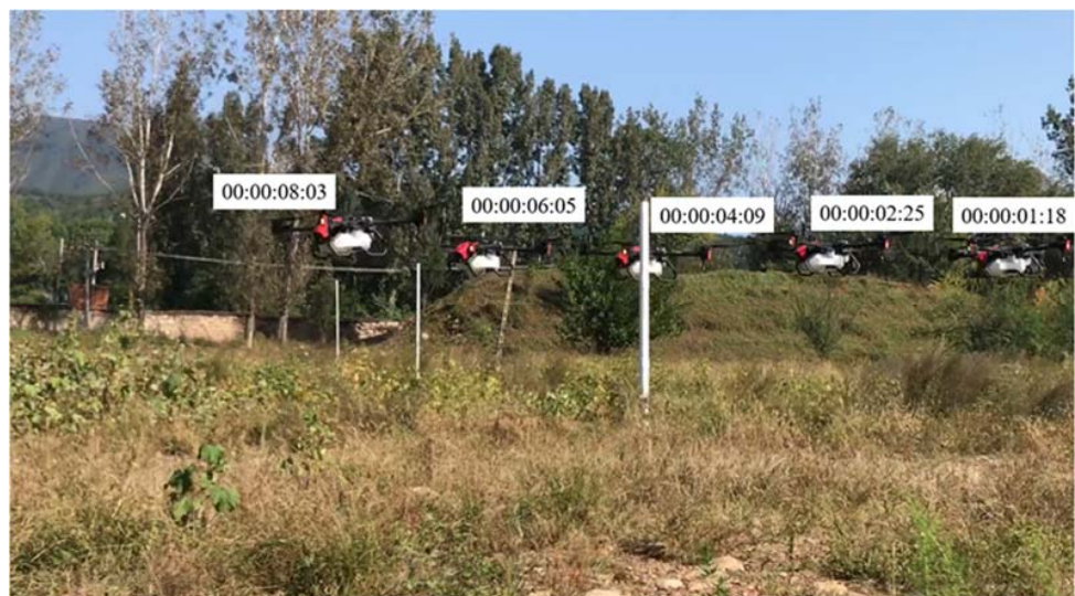
(a) Obstacle avoidance test of large-sized PVC pipe of XAG P80 (4 m/s)
