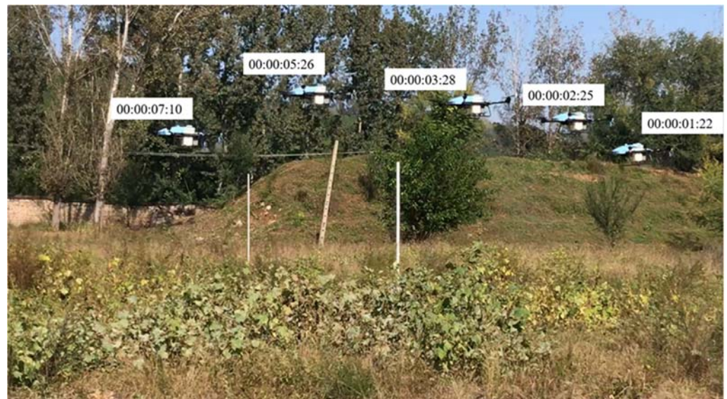
(a) Obstacle avoidance test of EAVISION E-A2021 in medium-sized PVC pipe (2 m/s)
