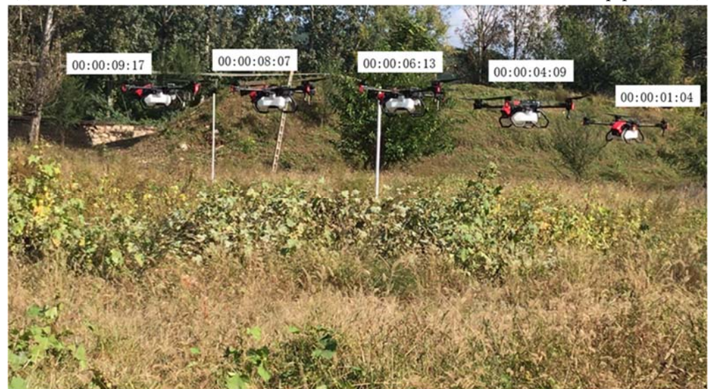
(b) Obstacle avoidance test of XAG P80 in medium-sized PVC pipe (2 m/s)
