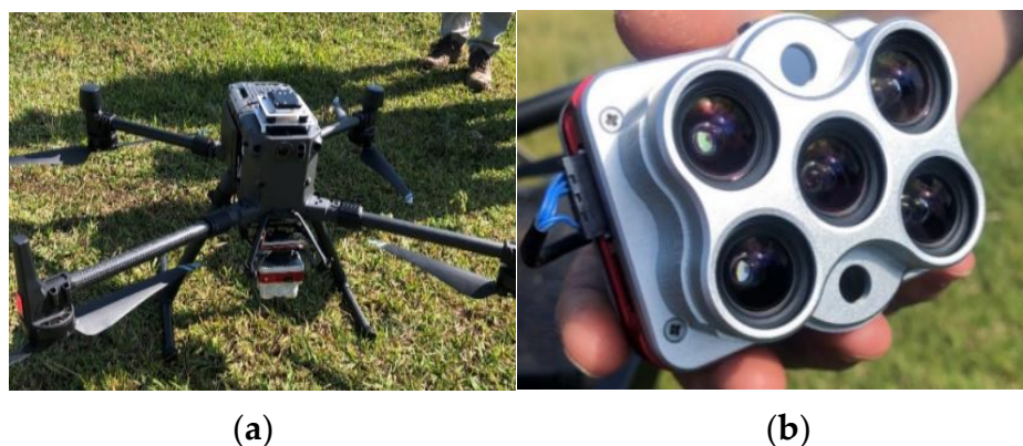
Figure 4. (a) DJI Matrice 300 platform and, (b) MicaSense Altum optical and thermal camera.
