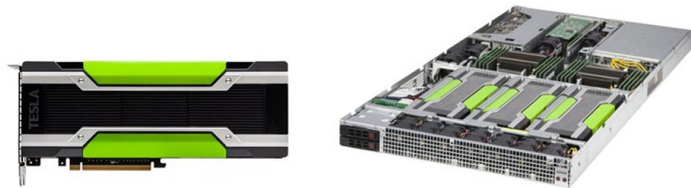
Figure 8. High-performance parallel computing server based on TESLA K80 parallel computing unit.
