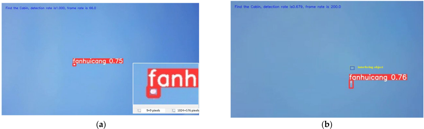
Figure 15. Target capture size and robustness. (a) The smallest size. (b) Detection with interference.
