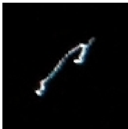
Figure 1. A region of interest containing a single star trail, captured from a strapdown celestial imaging sensor (Pi Camera HQ, 500 ms exposure interval). The shape of the star trail indicates that the camera was subjected to significant changes in attitude throughout the exposure interval.
