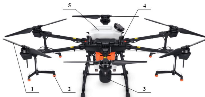
Figure 3. DJI T20 series plant protection UAV. (1) represents the propeller, which provides lift, (2) represents the nozzle, the droplet atomization device, (3) represents omnidirectional radar, which senses obstacles, (4) represents D-RTK, which is used for localization, (5) represents tank, which is used to hold the pesticide solution.
