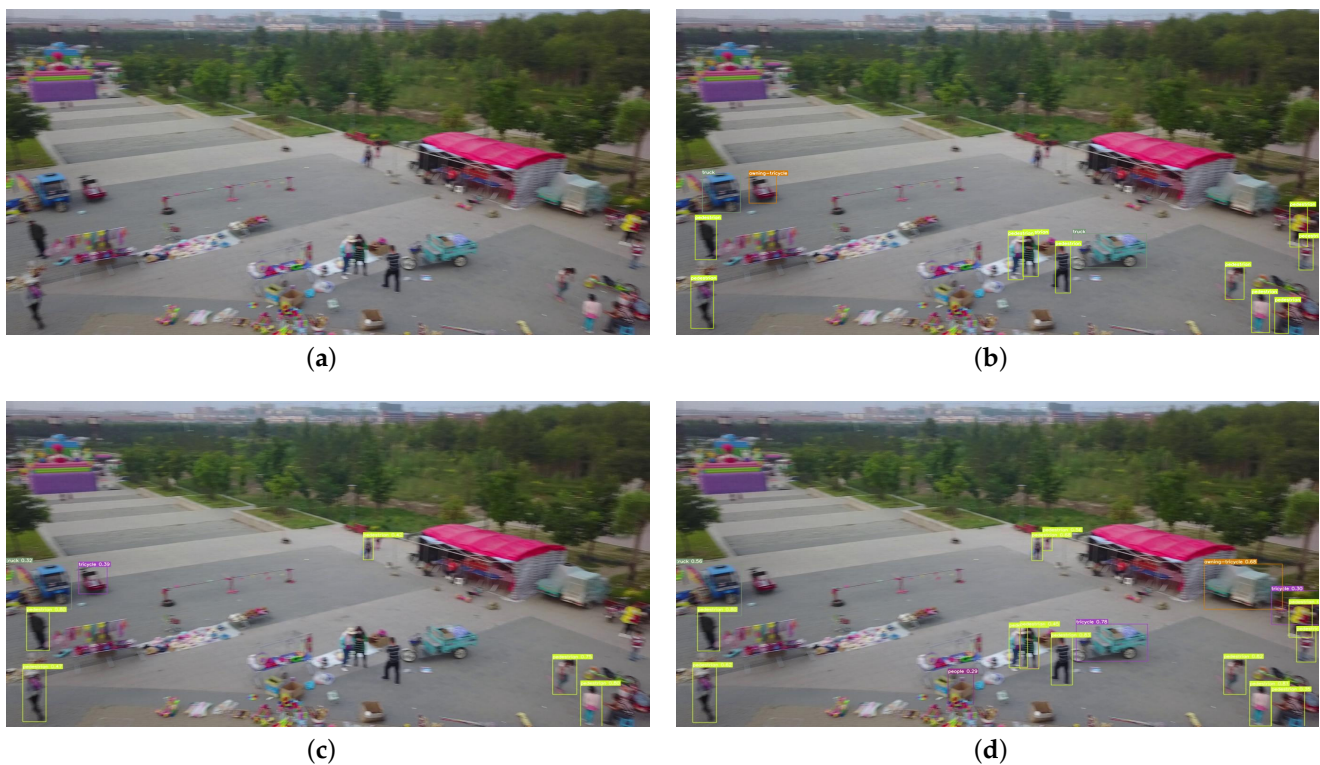
Figure 13. Detection results of YOLOv7 and SODCNN in motion blur scene. (a) Original input image. (b) Ground truth image. (c) Detection performance of the original YOLOv7. (d) Detection performance of SODCNN.
