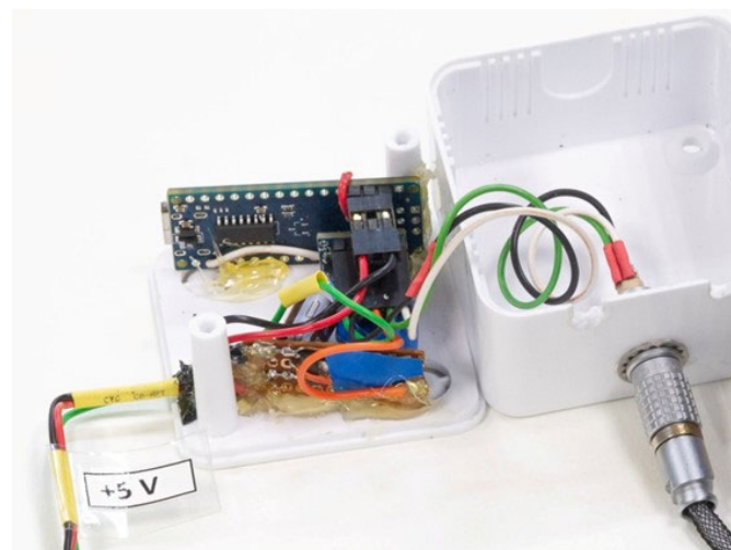
Figure 5. Internal structure of the LaserHub+.
