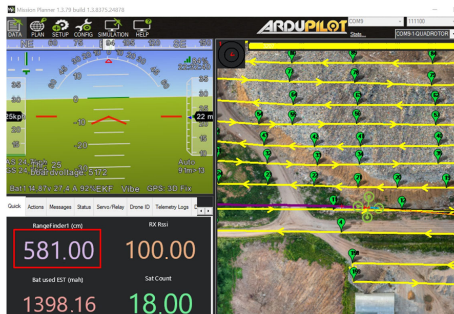
Figure 7. Display of the LMm detector readings in the Mission Planner program interface (highlighted with a red frame). The operation of the laser altimeter is emulated; the readings of the methane detector with a dimension of ppm*m are denoted with a dimension in cm.
