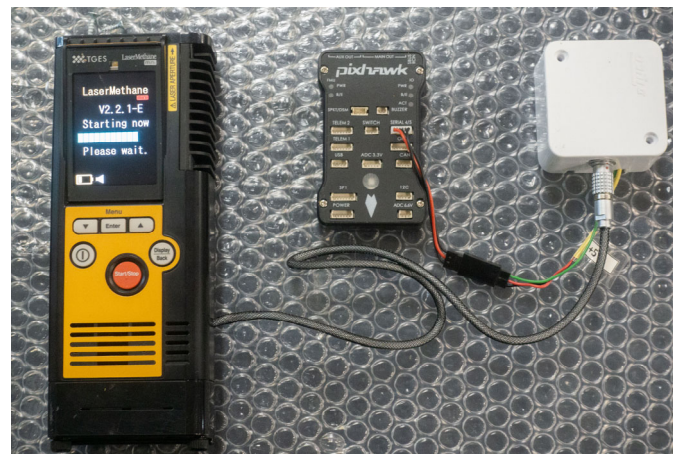
Figure 6. Connecting the LMm detector to the Pixhawk flight controller via the LaserHub+ device (on the left); LaserHub+ internals (on the right).
