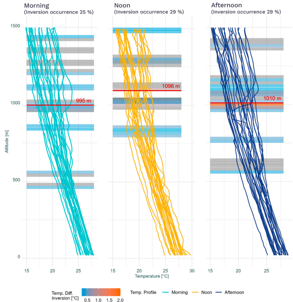
Figure 3. Microscale temperature inversions are characterised by a temperature rise of \geq 0.16 °C between adjacent 20 m altitude bins, progressing upward. A minimum of two consecutive layers of increasing temperature must be observed to be considered an inversion and further analysed. The weighted mean altitudes are computed based on the magnitude of temperature increases.
