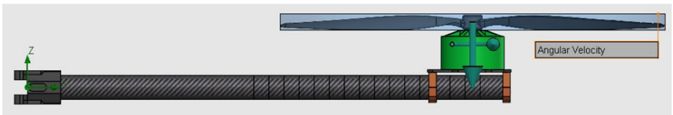
Figure 12. The region of rotation defined by the cylindrical volume surrounding the propeller area.
