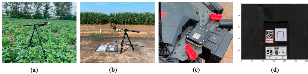
Figure 1. Acquisition of ground experiment images. (a,b) The camera configuration used to acquire reference images of the soybean field (a) and the calibration correction reference panel (CRP) (b). (c,d) Example images of a downwelling light sensor (DLS) mounted on an unmanned aerial vehicle (UAV) (c) and a CRP with barcode (d).
