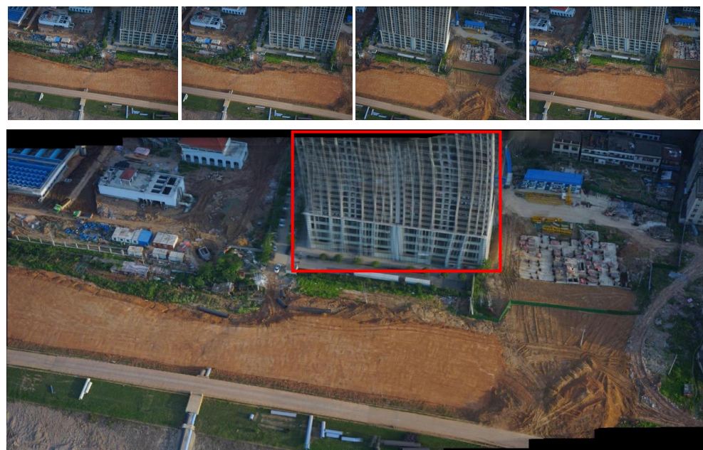
Figure 16. The failure case happens when the dominant plane cannot well represent the perspective transformation between images. The red box highlights the misalignments.
