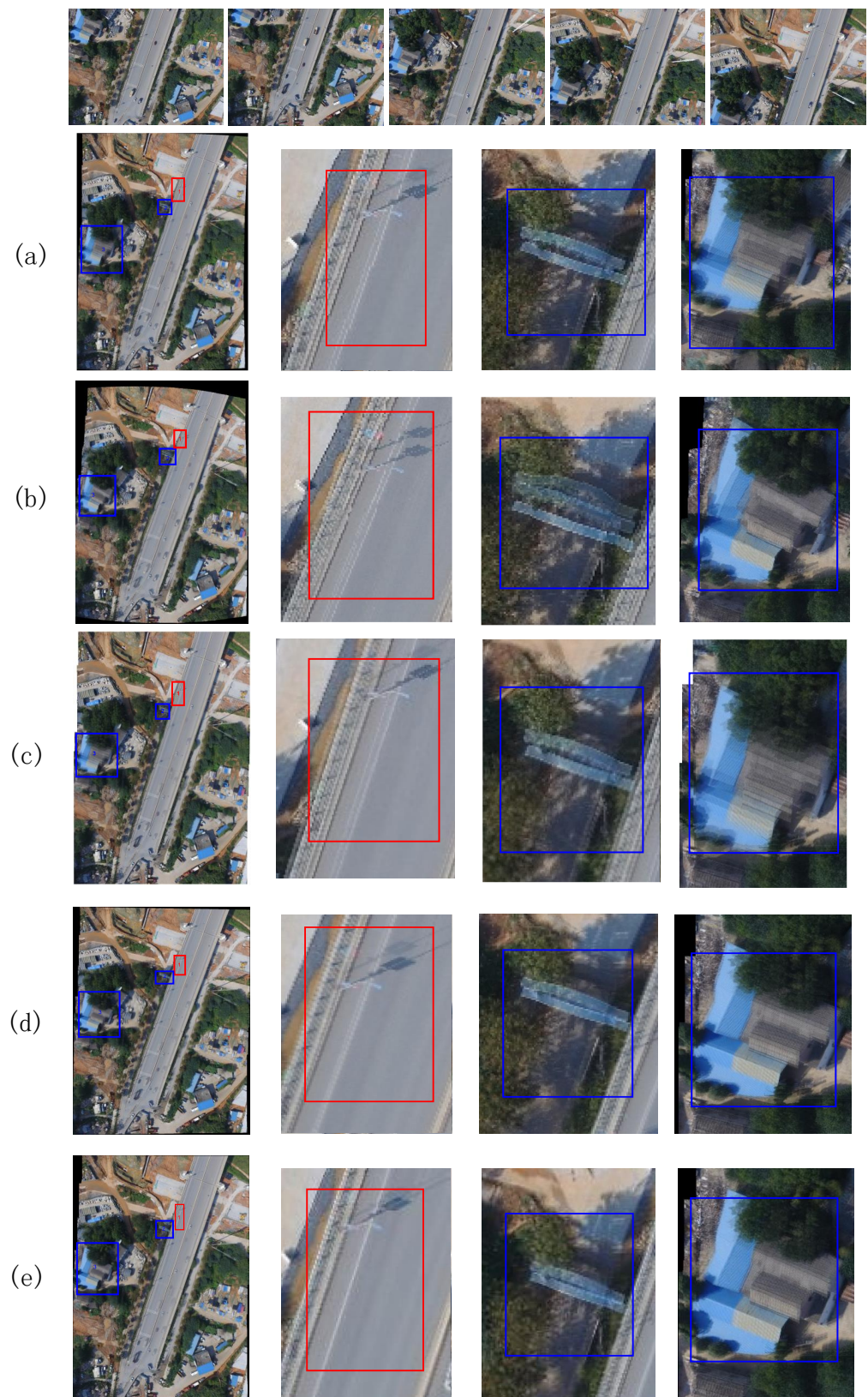
Figure 12. Qualitative comparison of alignment accuracy. From top to bottom, the first row is the input image, the others are the stitching results of (a) AutoStitch [22], (b) APAP [24], (c) SPHP [27], (d) SPW [36] and (e) our proposed method, respectively. For clearer comparison, we enlarge some areas and place them on the right side of the stitching results. The red box highlights the line alignment, and the blue box highlights the point alignment.
