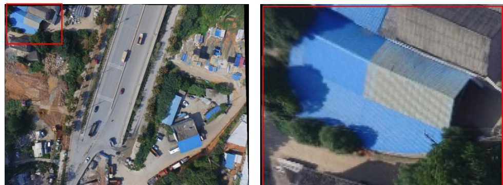
Figure 4. Illustration of bending of line segments due to the local mesh alignment. (Left) Warping result of local mesh alignment of one image. (Right) The enlarged area of the red box on the left image which explains the bending effect on line segments of local mesh alignment.
