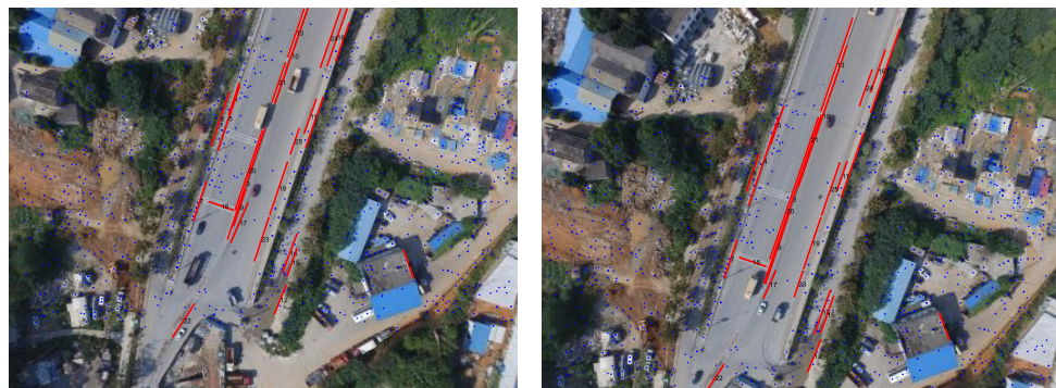
(a) Matching points and line segments on reference image and target image respectively
