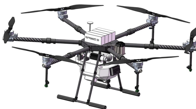
Figure 8. The 3D model and the layout design of the ecological plant protection UAV.
