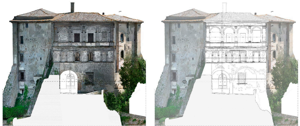
Figure 13. The two versions of the facade: on the left, the 2D representation overlaying the orthophoto at 100% opacity; on the right, the redrawn facade with a white background and the orthophoto at 60% opacity that completes the rest of the facade. The double representation was necessary to appreciate the quality of the details of the 2D drawings, which were the basis for an initial mapping of materials for the subsequent restoration project requested by the client, which analyzes degradations and interventions. At the same time, the full-opacity representation also makes it possible to appreciate the detail of the orthophoto in its material details (images by the authors).
