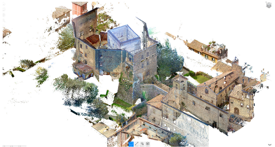
Figure 10. Point cloud processed in Autodesk ReCap from the laser scanner survey. The alignment of the scans starts from a master station which controls the entire project, to which the subsequent scans begin their alignment. The process is a progression: the second aligns with the first, the third with the second, and so on. Sometimes the source and destination scans need to be set manually, especially if the survey does not follow a chronological order, as often happens. The overlap is done automatically, or by indicating three pairs of points on two different scans (image by the authors).
