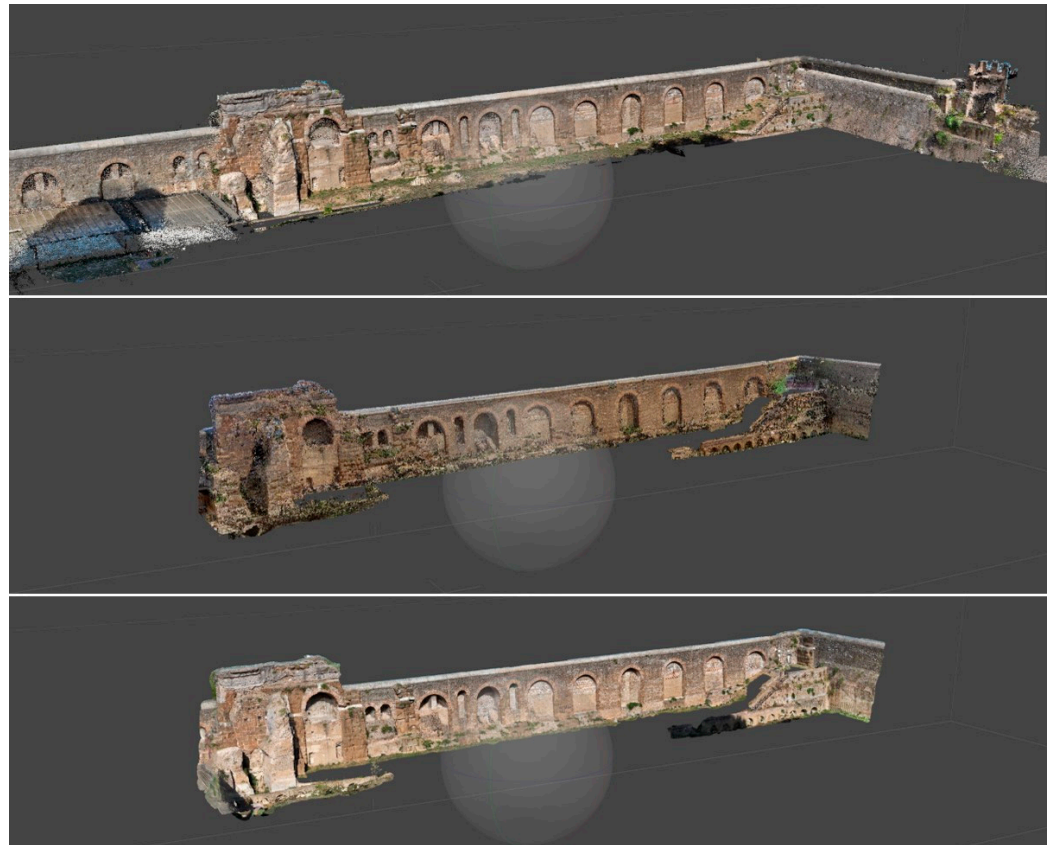
Figure 22. The dense laser scanner point cloud was exported from CloudCompare with the new Cartesian position coincident with the lower-quality drone point cloud. This way, it was possible to import the laser cloud into the Metashape source file, in the same position, and proceed to the creation of a mesh model more detailed than one from SfM. The 3D model finally underwent the texturing process, exploiting the photos taken by drone. From the top: dense point cloud from drone survey; dense point cloud from laser scanning; laser-scanner-derived mesh, textured by the drone survey (images by the authors).
