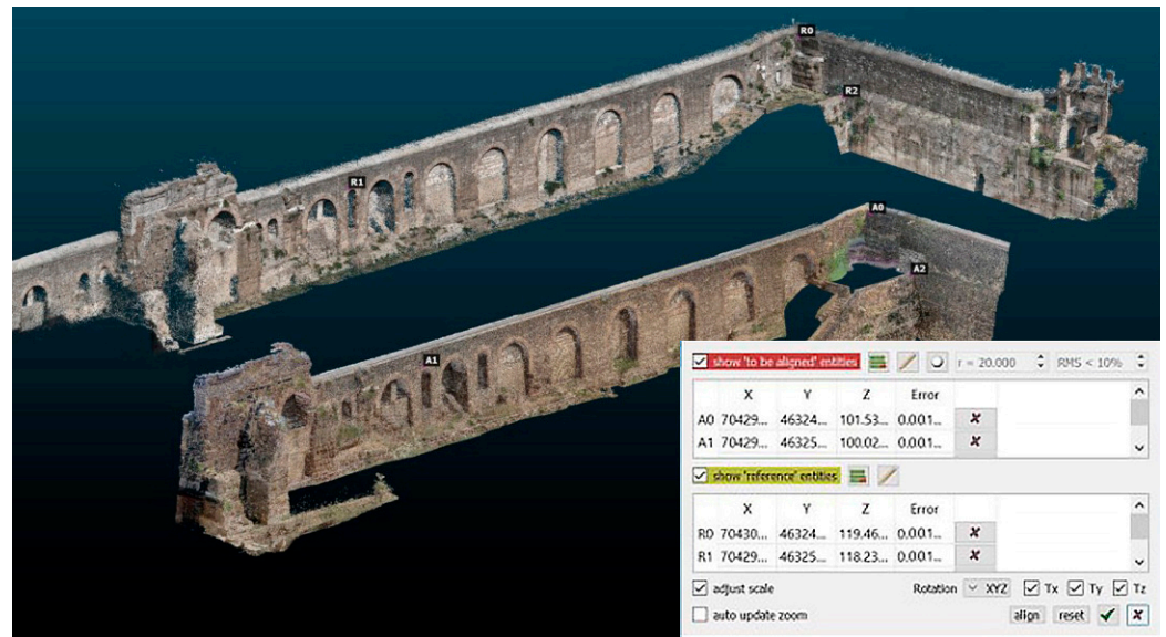
Figure 20. Selection of common points between the two imported point clouds in CloudCompare. The choice of targets for the alignment of the two point clouds must be such as to guarantee some characteristics: the points must be rather distant, to avoid a specific scaling and rototranslation in favor of a general one (in this case, for example, the length of the aqueduct); the points must belong to at least two different and/or orthogonal planes, preferably on the three Cartesian planes (image by the authors).
