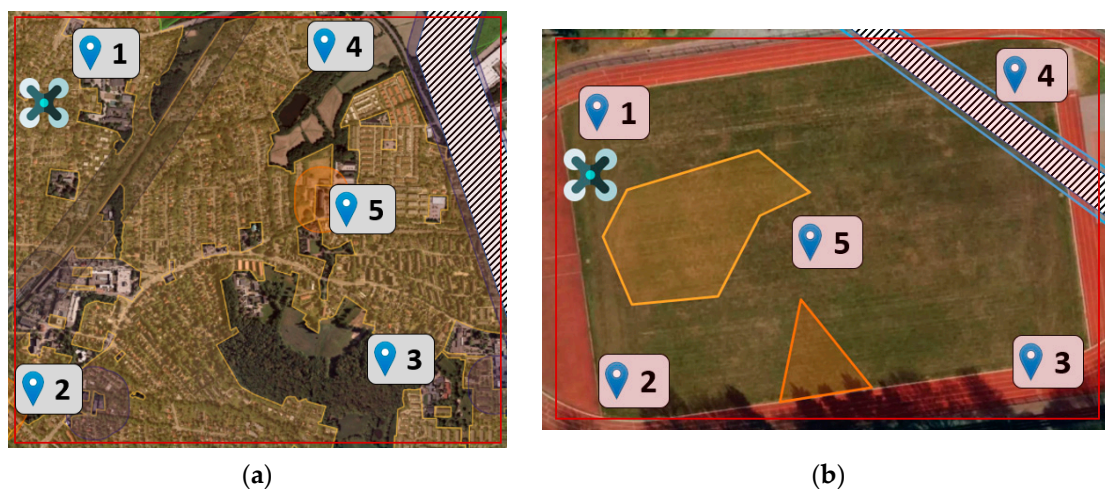
Figure 3. Top view of the presented missions showing the position of the UAV, goal locations, the environment, geographical zones and the geofence for the simulation-based mission M1 (a) and the real-life mission M2 (b).
