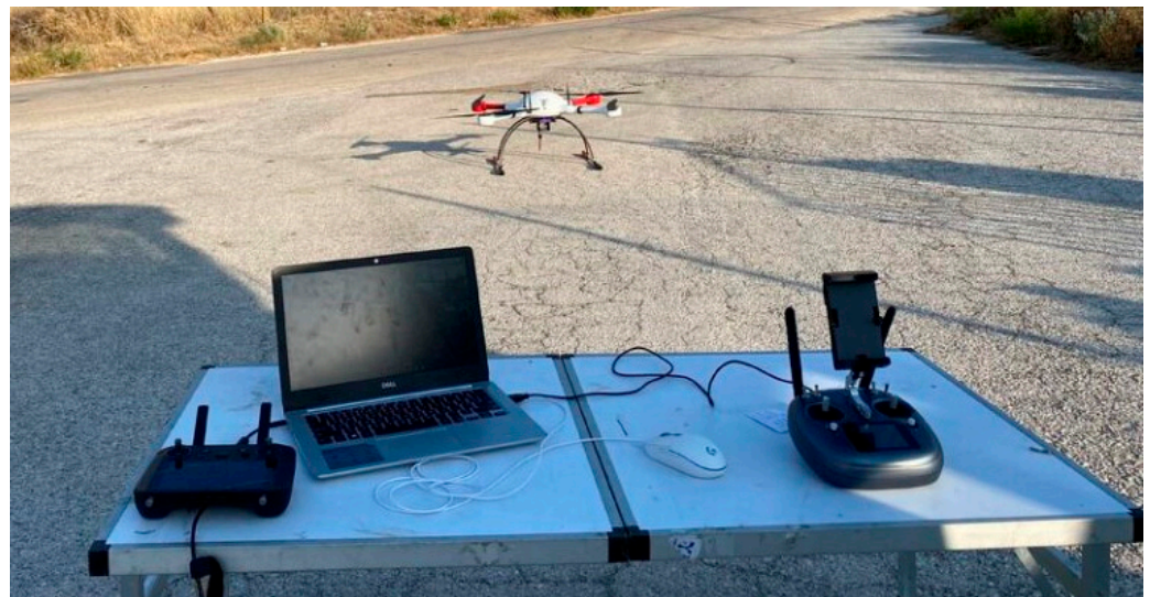
Figure 2. Field setup of the ground control station, the controller, and the cargo drone.
