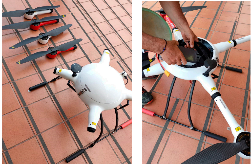
Figure 1. Cargo drone assembling: (left) airframe body and four fixed propellers and (right) battery fastening.
