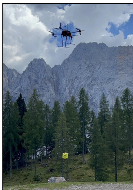
Figure 3. AED hanging on a 5 m rope attached to the drone. Source: The authors.
