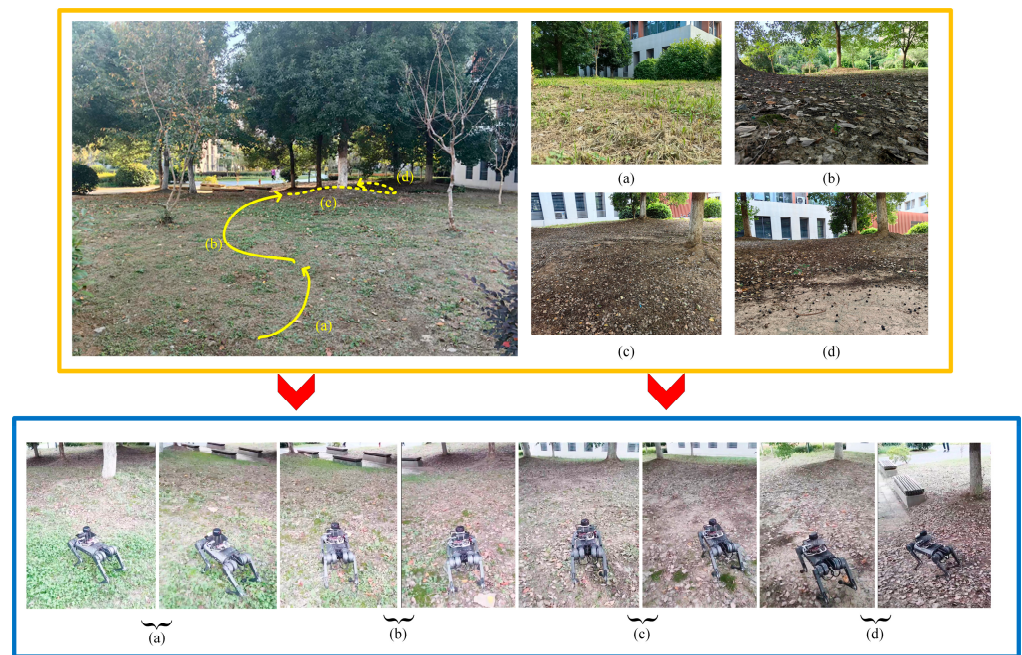
Figure 26. Demonstration of experimental robot walking routes in complex outdoor environments. (a–d) represent the 4 parts of the S-curve respectively.
