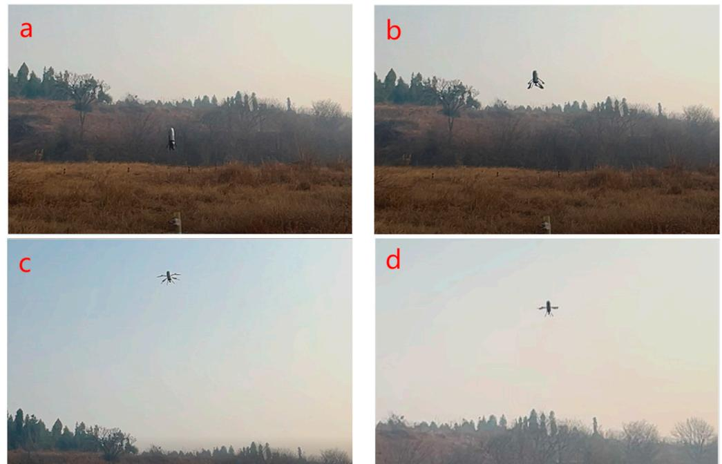
**Figure 12.** Static experiments on the barrel launching process. (a) The launch barrel phase; (b) the spread arm phase; (c) the attitude control phase; and (d) the climb rate control phase.
