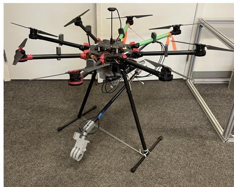
Figure 5. Aerial vegetation sampler experimental platform.
