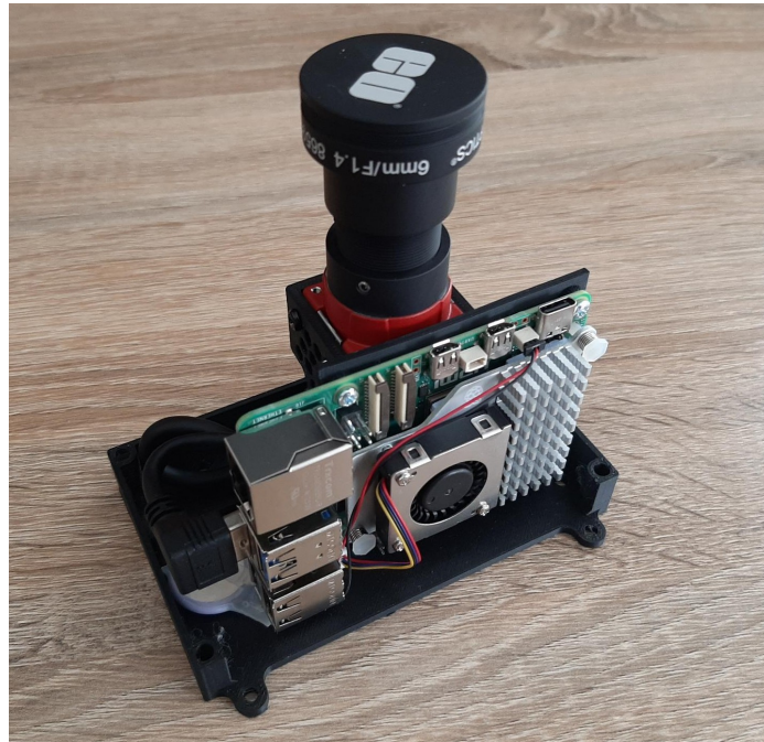
Figure 4. The celestial payload, consisting of a Raspberry Pi 5 and an Alvium 1800 U-240 monochrome sensor fitted with a 6 mm f/1.4 wide angle lens.
