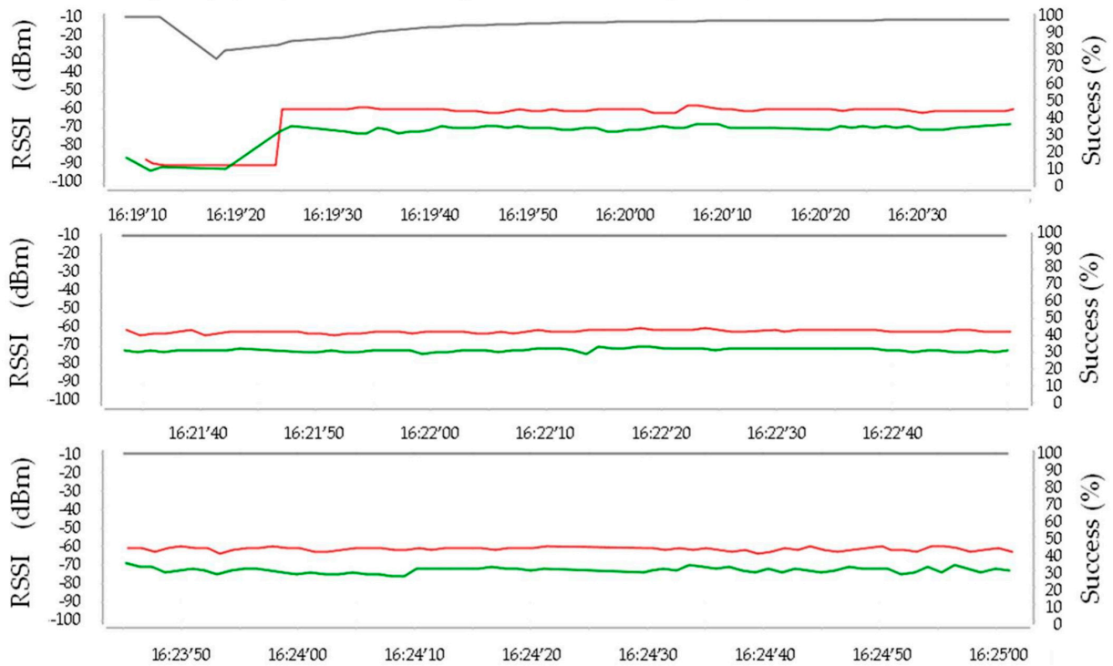
Figure 16. Results of range tests with a hovering relay drone positioned at the center of a 100 m line of sight. RSSI: Received Signal Strength Indicator. Success (%) on the right-side vertical axis represents the Packet Delivery Ratio (PDR, %). The test for each condition was repeated three times. Each packet was to be sent ideally at 1000 ms intervals, but the receiver timeout was set as 10 s for a measurement of water quality at 10 s intervals. The average PDR was 97 \pm 2.7\% for the on-ground relay and 100 \pm 0.3\% for the hovering relay. The sensitivity of the receiver (XBee™ S2C coordinator in the boost mode) was -102 dBm [17].
