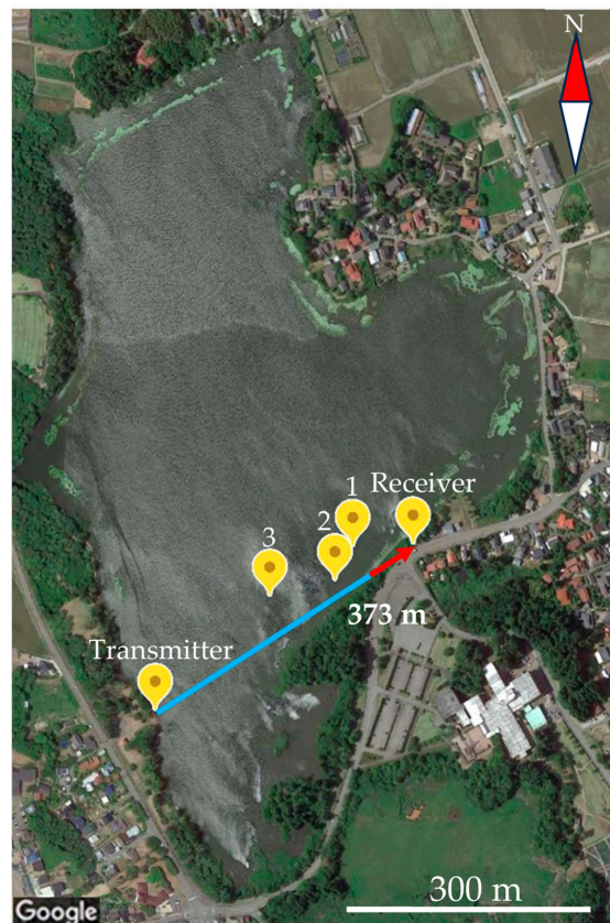
Figure 19. Locations of wireless water quality monitoring system for bypassing relay test (Ogata Pond on 27 September 2022): Transmitter, transmitter drone (landed on the water and was fixed by mooring from shore); 1–3, locations where the relayer drone was placed; Receiver, receiver on a tripod. Red arrow indicates the wireless communication path blocked by shoreline vegetation.
