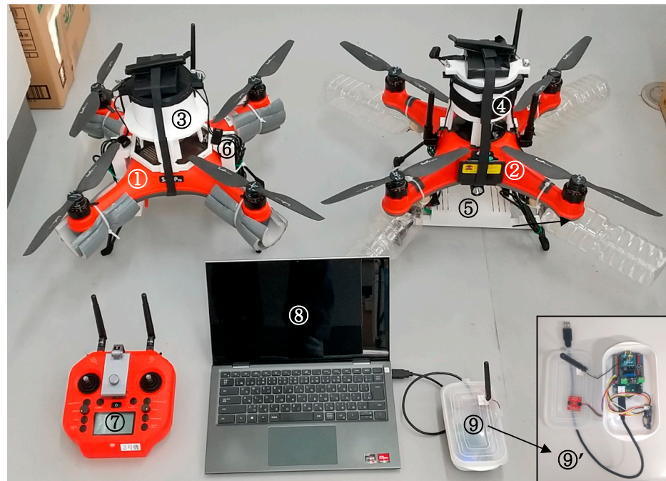
Figure 9. Components of the water quality monitoring system with amphibious drones for wireless data relay tests: 1, SplashDrone™ 3+; 2, SplashDrone™ 4; 3, upper mounter for SplashDrone™ 3+; 4, upper mounter for SplashDrone™ 4; 5, lower mounter for SplashDrone™ 4; 6, side mounter(s) for SplashDrone™ 3+; 7, drone controller for SplashDrone™ 4; 8, laptop computer for data display; 9, receiver; and 9', contents included in the receiver.
