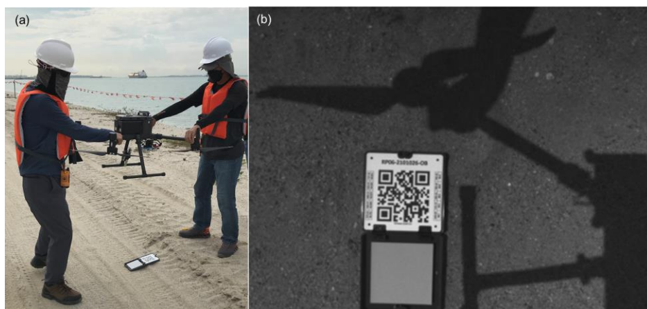
Figure 5. Demonstration of the standard position for the DJI M300 RTK—Micasense Rededge-MX Duo with (a) the camera at 1 m above the reflectance panel and (b) the placement of the panel with no shadows cast on its surface.
