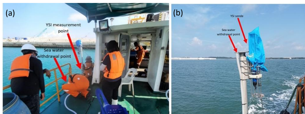
Figure 14. Placement of the YSI probe and seawater pump (a) with a 2 m gap (before April 2022) and (b) on a steel pole with a 50 cm gap (from May 2022 onwards).
