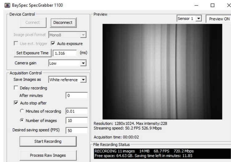
Figure A1. Example of SpecGrabber GUI software for Bayspec camera settings prior to UAV operations with the manual adjustment of exposure time.
