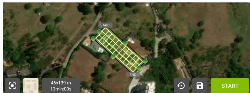
Figure 6. Flight plan over the study area at an altitude of 3.00 m (9.84 ft).
