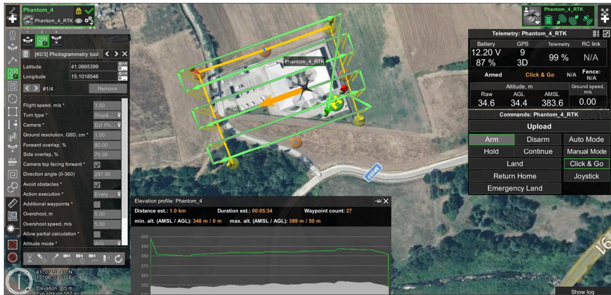
Figure 6. UgCS Enterprise v. 4.20 software interface for UAS mission planning. In the left panel are shown the set parameters for the flight plan; the right panel shows the UAS telemetry, and the bottom window displays the survey's altimetry and number of waypoints.
