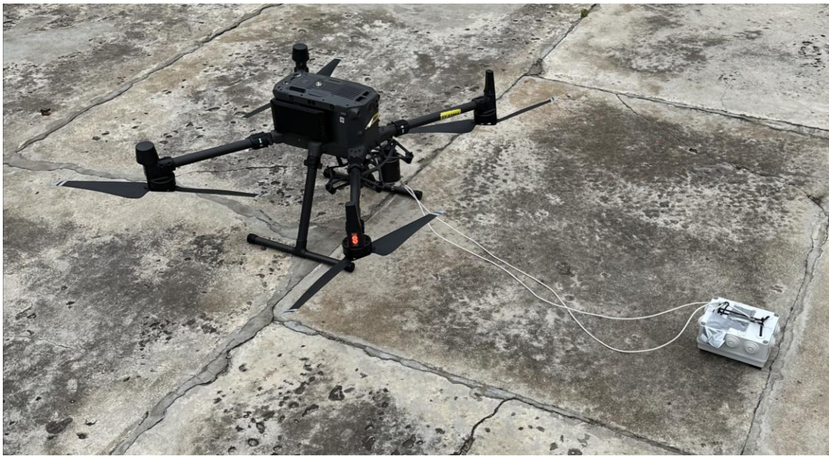
Figure 8. UAV test for the SSM communication link: drone and collar configuration.
