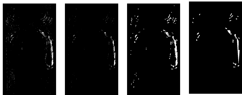
(a) Bilateral filtered (b) Erosion (c) Dilation (d) Contour approximation
