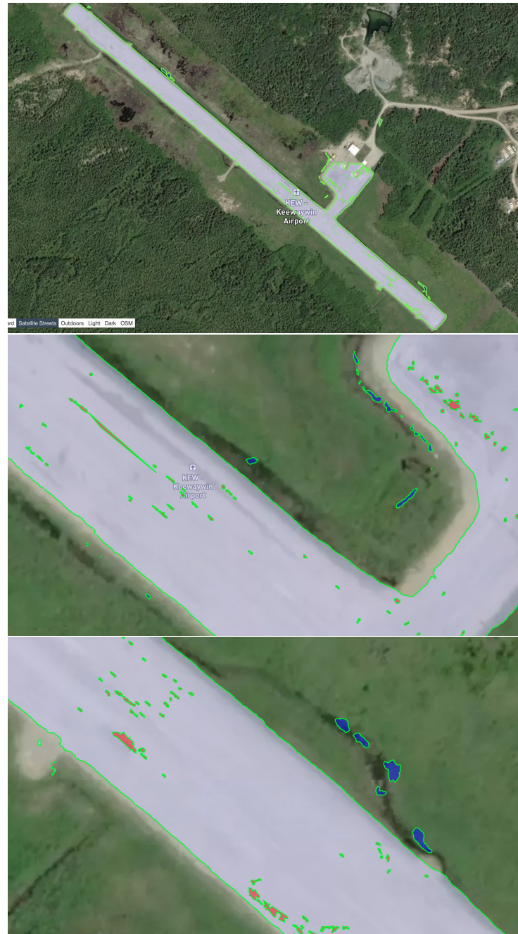
Figure 11. Visualized results overlaying a satellite map. The bright green contours highlight all detected targets, including runways, vegetation, water, and rough surfaces. They are distinguished by various filling colors, e.g., runway as purple, water as blue, vegetation as green, and rough surfaces as red.
