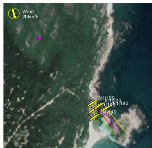
Figure 6. UAV swarm reaches a V-shaped formation.
