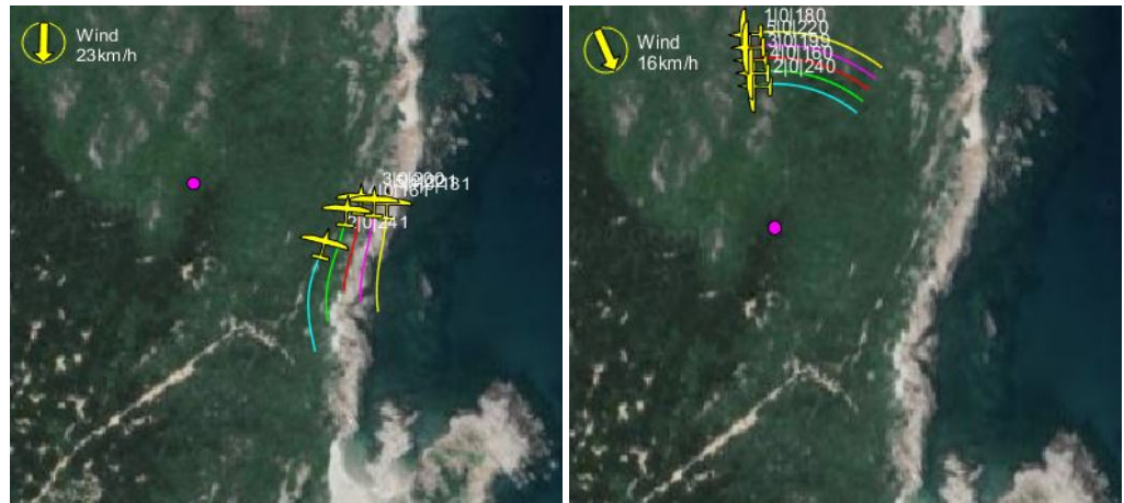
(a) UAVs' positions before reaching loitering (b) UAV swarm reaching loitering formation Figure 7. Evolution of UAVs' positions.
