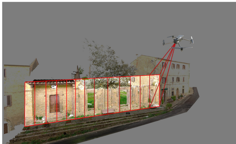
Figure 5. UAV collecting church data.
