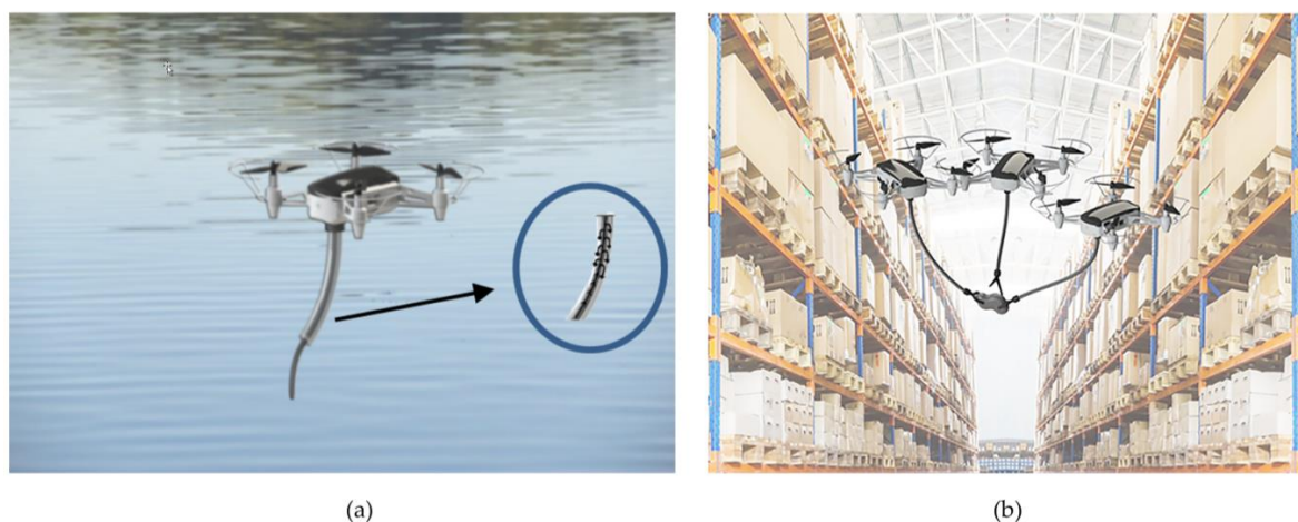
Figure 2. Two different contexts of application of CAAMS: (a) water sampling, (b) cooperative manipulation. Reprinted/adapted with permission from [31], 2022, Farrokh Janabi-Sharifi.
