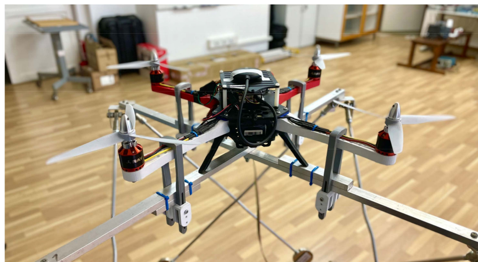
Figure 15. Drone attached to the measurement system.
