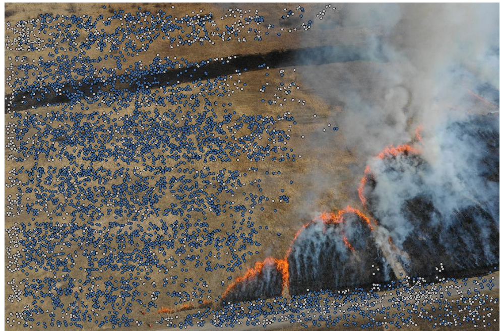
Figure 11. Example of the distribution of tie points used for orienting the selected image. Blue points represent those for which a corresponding pair was found in subsequent images, while gray points represent those for which no match was found.
