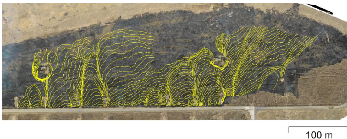
Figure 10. Result of manual vectorization of fire spread at an 8 s interval. In the background is an orthophoto mosaic of the burned meadow from the last flight.
