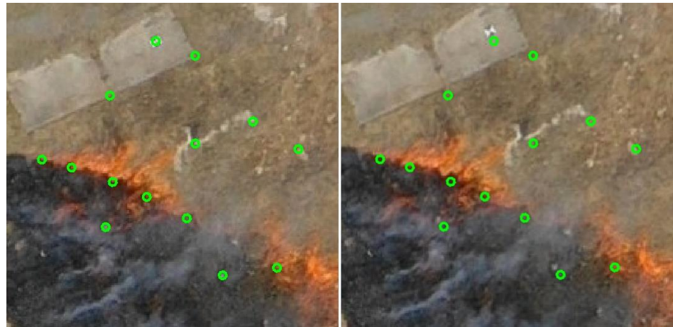
Figure 18. Detail of the orthoimage rectified based on the 3D model from the post-fire flight ( left ) and the deformed model generated from the side monitoring flight ( right ). Differences in the position of the green markers against the background texture are visible in the images. Deviations reached a maximum of 0.3 m, which corresponds to the vertical deviation of the model in the corresponding area in Figure 14.
